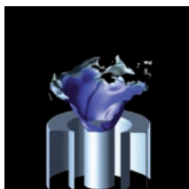
The G=0 illustrates the flame front where the colour represents the equivalence ratio having its maximum value at inflow ( =0.833 )
